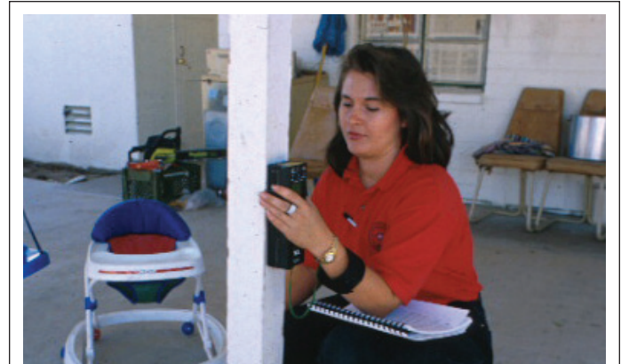
FIGURE 7.7 Lead inspectors should operate XRF instruments at a safe distance from others.
